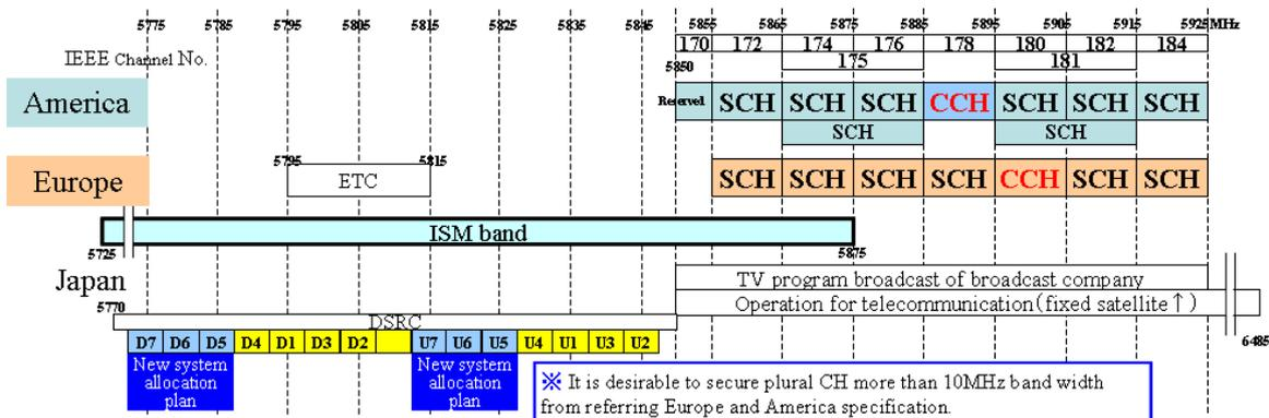
Figure 1. DSRC frequency allocation for Japan, Europe, and America, and new communication system CH allocation example.
